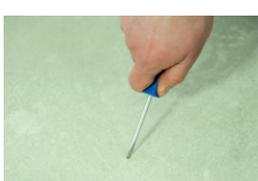
The glue-down procedure should only be used with concrete grades 3,000 psi or higher. Glue-down installation on lightweight concrete (less than 3,000 psi) is not permitted. Always perform the glue bonding test before starting glue-down installation.
